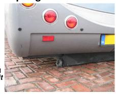
How it works: this auxiliary or helper spring kit has two specially designed brackets, fitted on the AL-KO chassis and suspension arm. Two very long steel coil springs of 350/380mm length are placed in between. Because of the small
